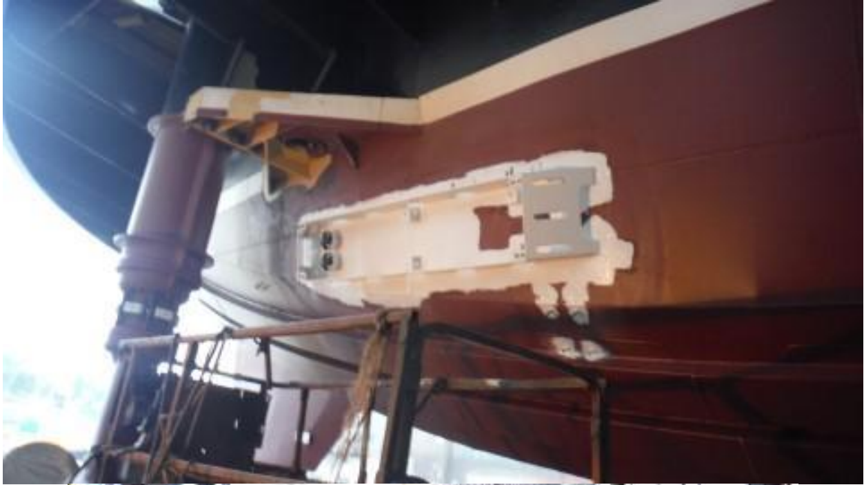
Detail of new Fernstrum® keel cooler frame.
