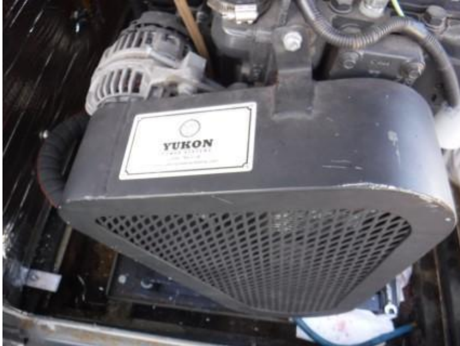
Detail of new ship service generator and sound enclosure.
