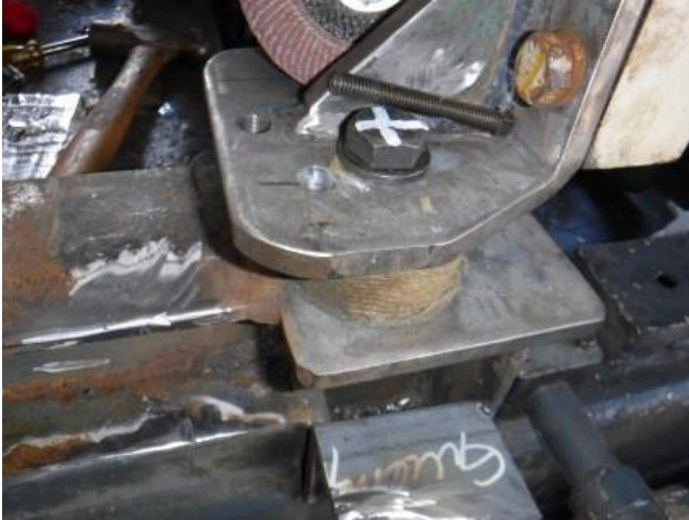
Detail of Vibracon propulsion engine mount
